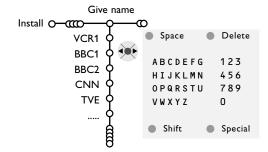
It is possible to change the name stored in the memory or to assign a name to a TV channel or external for which a name has not yet been entered. A name with up to 5 letters or numbers can be given to the programme numbers 0 to 99 and to the externals.
